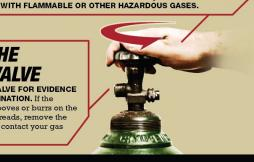
Also referred to as "cracking the valve." SLOWLY OPEN THE CYLINDER VALVE AND THEN IMMEDIATELY CLOSE IT to blow out
