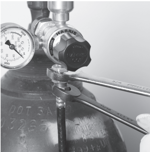
Figure 3. Attaching Hose to Flowmeter/Regulator
